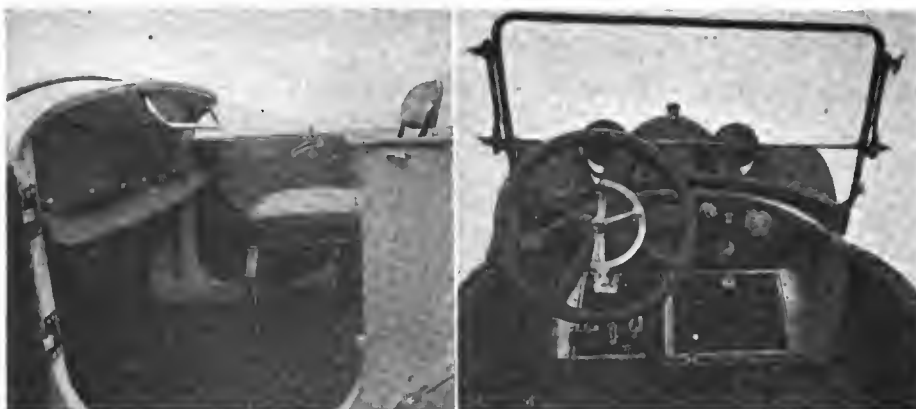
Left—Tonneau, showing compartment into which auxiliary seats fold. Right—View of cowl and control showing the arrangement of the levers—the brake lever is set forward out of the way and the ball-handled gear lever is placed between the seats
